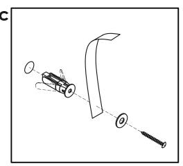
Attach Tipping Restraint to the wall using 1 1/2" Round Head Screw, Flat Washer (Large) and Anchor.
