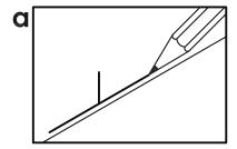
Place the unit on the wall at desired location. Mark with pencil to show the height and center of unit.
