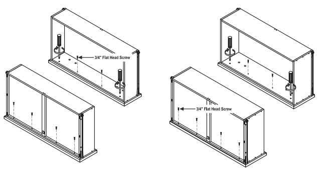
Note: These 3/4" Flat Head Screws on this page must be installed to complete the drawer assembly.
