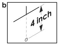
Move unit. Drill a 1/2" hole in the wall, 4 inches down and directly below the mark.
