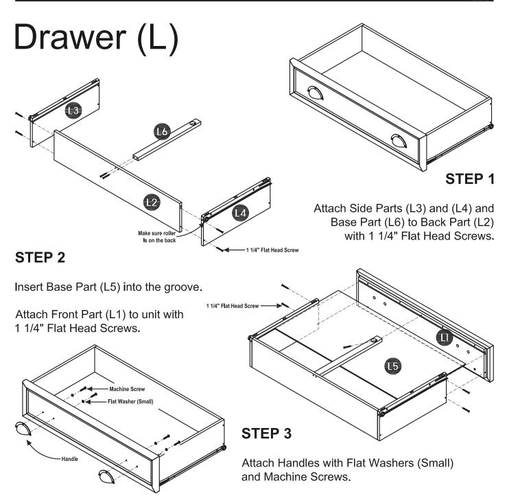
Note: Drawer assembly is not complete until 3/4" Flat Head Screws are used in a later step.
