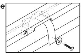
Screw Tipping Restraint to unit using 1/2" Round Head Screw and Flat Washer.
