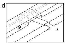
Insert Tipping Restraint to unit through the groove of Top (A).
